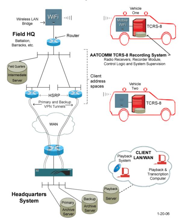
In an enterprise-wide system, the TCRS Companion Intermediate Servers located at each field headquarters, battalion or barracks may be networked via a LAN/WAN or protected Virtual Private Network to a fully redundant Centralized Archive and Playback System – C.A.P.S. - as shown above. C.A.P.S. systems are accessible for search, retrieval, playback and transcription activities using an intuitive remote access software application residing on client provided desktop computers.
