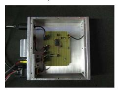
With a "one-off" design, a device like the Universal XTL-5000 radio interface must be custom engineered and handwired as seen to the left.
