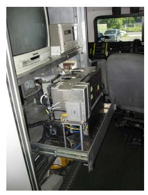
The original TCRS-8 Main Electronics Unit includes provision for eight (8) Motorola XTL-5000 UHF radios. For the FCU, in the space formally occupied by the eighth radio, a custom interface was provided to the externally mounted 800MHz. trunking radio:
